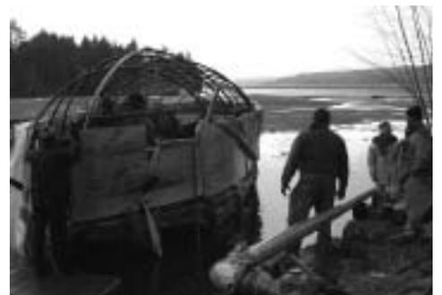
When the ice went out at Basin Harbor, caulking was dislodged, and our pump could not keep up with the incoming water. For two days our dive team worked in 36-degree water to caulk the seam, attach plywood around the sides of the boat, and pump her out, with the able assistance of LCMM Trustee Bob Beach and the Basin Harbor Club crew.
